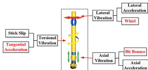
Fig. 2 Three main modes of downhole vibration [9]
