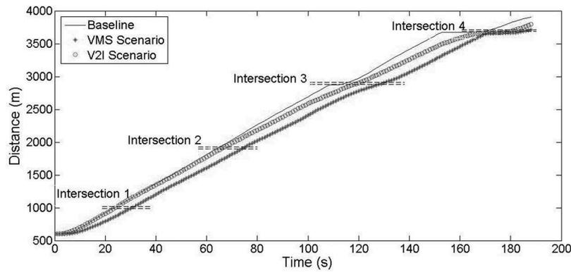
Figure 6. Driving trajectory of a vehicle crossing the four intersections in different scenarios.
