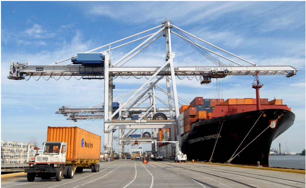
Figure 2.2: Ship-to-Shore Gantry Cranes (Source: Google Image)
