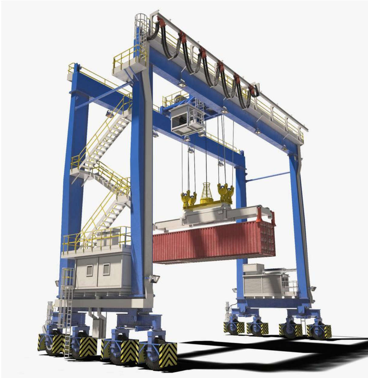
Figure 2.3: Rubber Tire Gantry (RTG) Crane (Source: Google Image/free3d.com)
