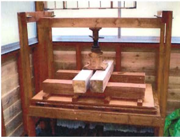
Figure 5. The Assaku , or the process of squeezing papers.
